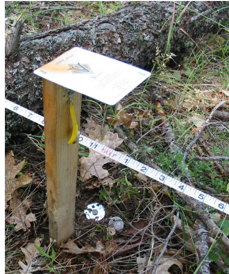
Figure 1. A monitoring station to measure aboveground temperature and relative humidity. On the surface of the ground to the right of the stake you can see the washer and tag for a belowground iButton.
