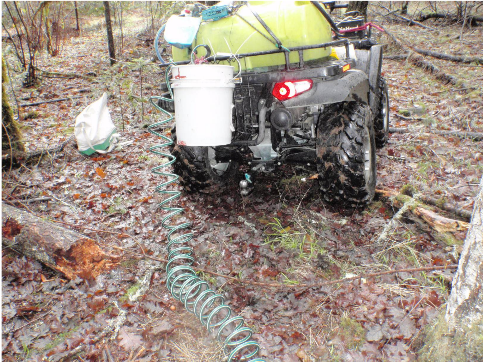
A garden spring-coil hose works suitably well also – but is harder to recoil.
