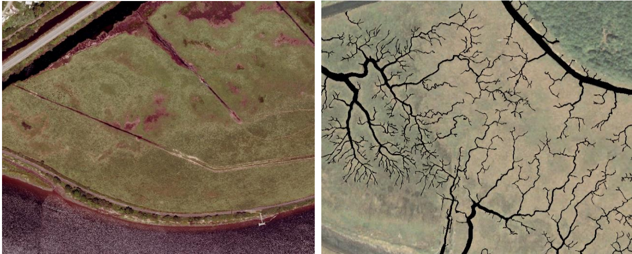
Figure 16. Channel network density comparison. Left: simplified channel (ditch) network in a 75 acre section of Waite Ranch. Channel density is about 0.02 mi/acre; channel length is about 1 mi. Right: dense, dendritic channel network in a 75 acre section of least-disturbed tidal marsh (Millport Slough, Siletz Bay NWR, surveyed by So et al. (2009). Channel density is about 0.15 mi/acre; channel length is about 11 mi. Figure from Brophy and Lemmer (2013).
