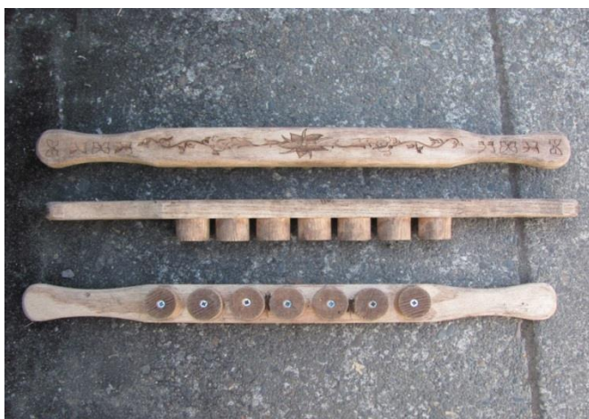
FIGURE 18: TOOLS SUCH AS SOIL TAMPERS HELP EVENLY PACK SOIL TO THE CORRECT LEVEL IN EACH CELL (PHOTO LARKIN GUENTHER)
