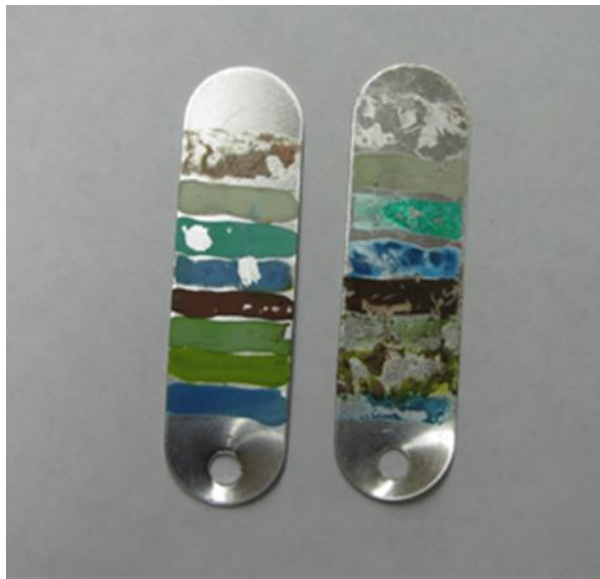
Figure 3. Temperature indicating paint on burned (right) and unburned (left) plot tags.
