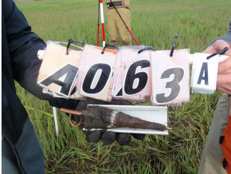
Figure 2. Example of field photo showing a feldspar marker horizon core and its sample number. This core shows an excellent quality feldspar layer. A photo like this was taken of each core, for archival purposes. Sediment to the left of the white feldspar horizon has been deposited since the feldspar layer was placed in 2013.
