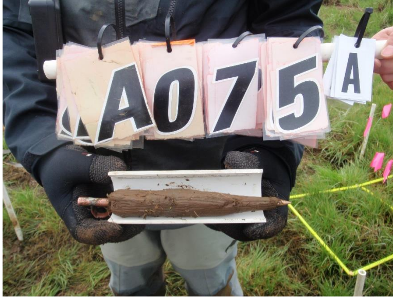
Figure 4. Example of field photo showing a feldspar marker horizon core with no visible feldspar layer. Cryocores lacking a visible feldspar layer typically occurred in areas dominated by reed canarygrass.
