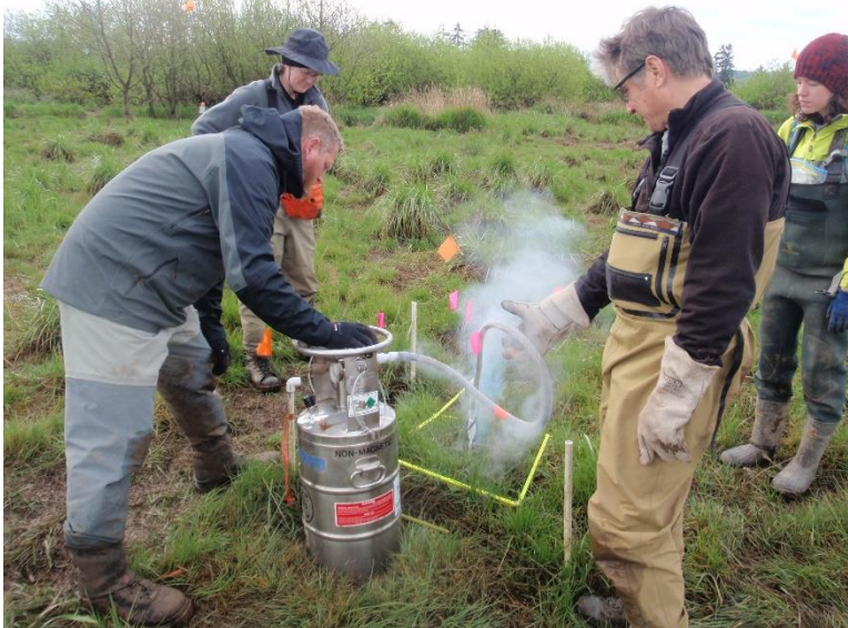
Figure 1. Field crew collecting cryocore at a feldspar marker horizon plot. Liquid nitrogen is injected into the ground through a small copper tube, which creates the frozen core that is removed for measurement (Figures 2-4).
