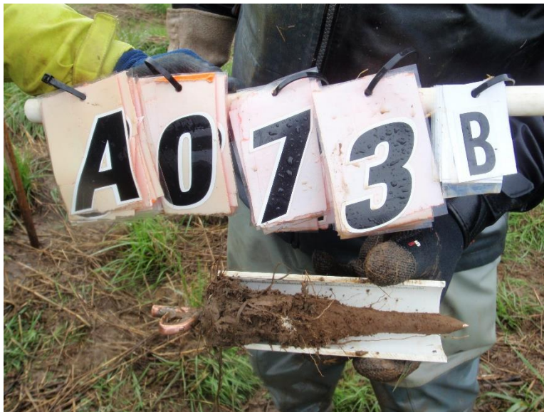
Figure 3. Example of field photo showing a feldspar marker horizon core with an incomplete or low-quality feldspar layer. Cryocores of this and lesser quality were common in areas dominated by reed canarygrass.
