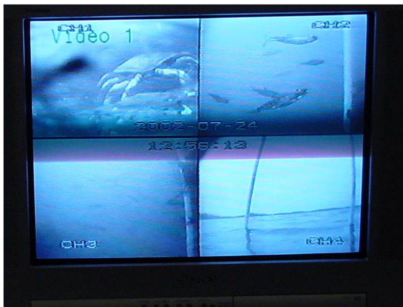
Figure 82. Example view of sampling data gathered using videography. The four views represent different cameras located at different elevations off the channel bed within the same sampling station (pole).
