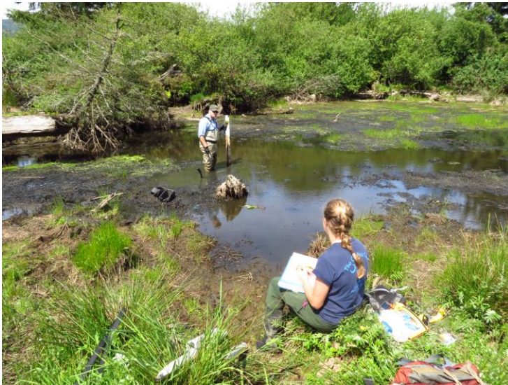
Figure B19. Michael Ewald (L) and Laura Brown (R) downloading the automated datalogger in upper Blind Slough. This logger was discontinued partway through the monitoring period due to low water. Photo by Laura Brophy.
