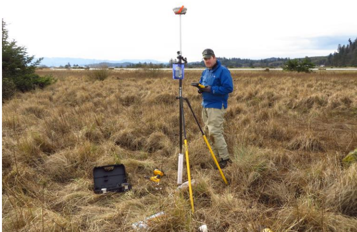
Figure B20. Michael Ewald measuring elevation of monitoring infrastructure using high-accuracy RTK-GPS equipment. Photo by Laura Brophy.
