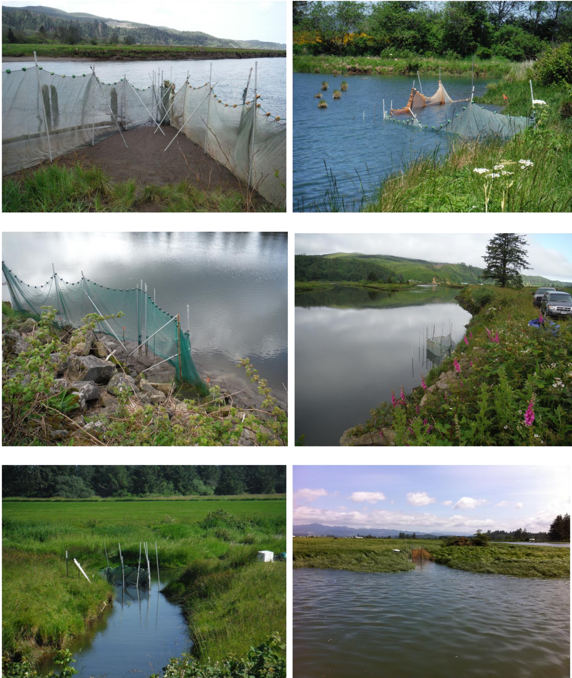
Figure B17. Photos of guide nets used to direct fish away from the shoreline, while concentrating migrants in front of sampling cameras at three reference and one SFC location.
