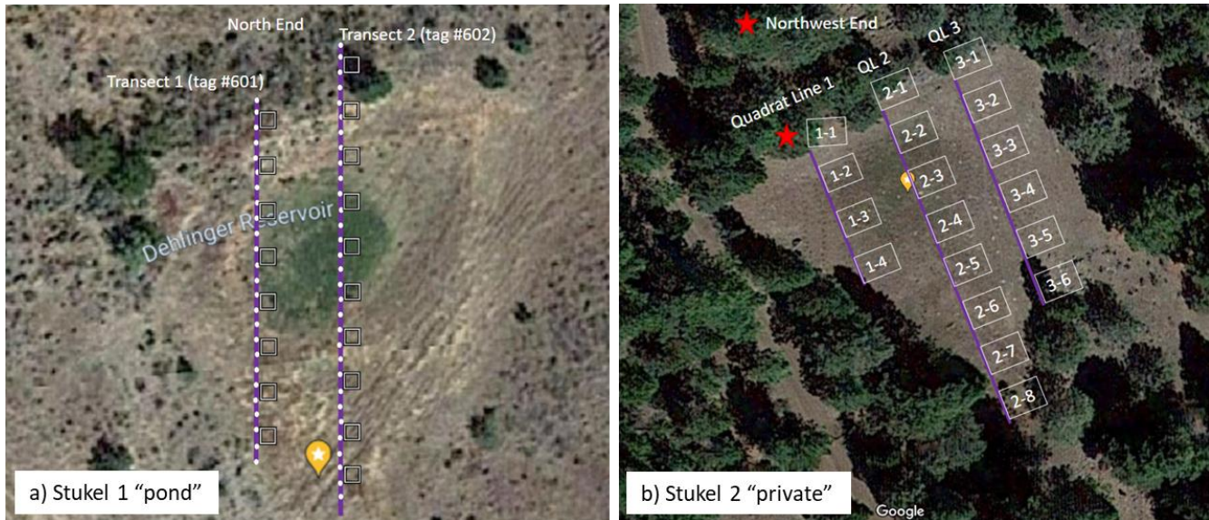
Figure 6. Diagram showing how two sites on Stukel Mountain, (a) Stukel 1 “pond” and (b) Stukel 2 “private”, were set up with transects (purple lines) and quadrats (white squares) to survey vegetation communities associated with Columbia yellowcress ( Rorippa columbiae ). The red star indicates that at the ‘private’ site, quadrats were angled slightly off the quadrat line to orient northwest-ward. Satellite imagery from Google; diagrams are representative and not drawn to scale.
