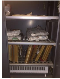
dry heat (57°C/5% RH) in the herbarium specimen drier for five days
