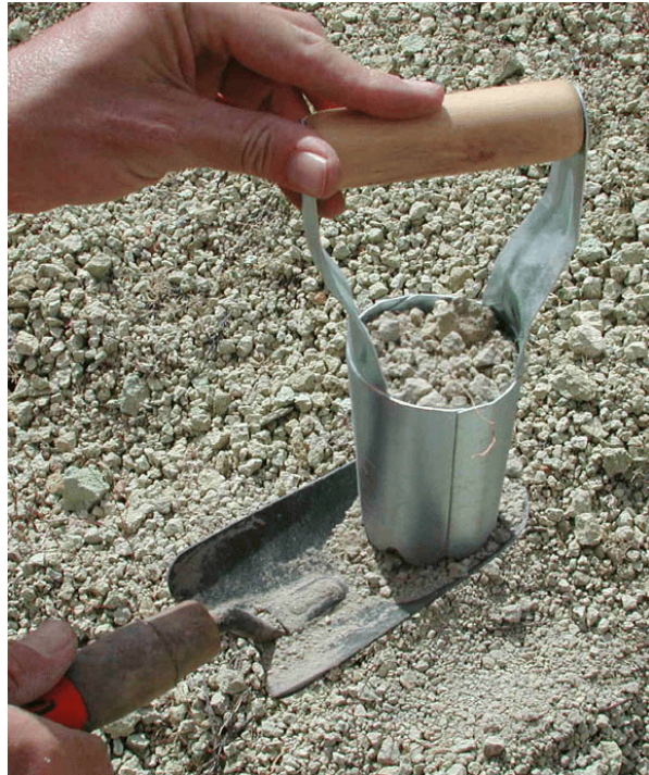
Figure 9. Photograph showing collection of soil core samples within S. erterae research plots.
