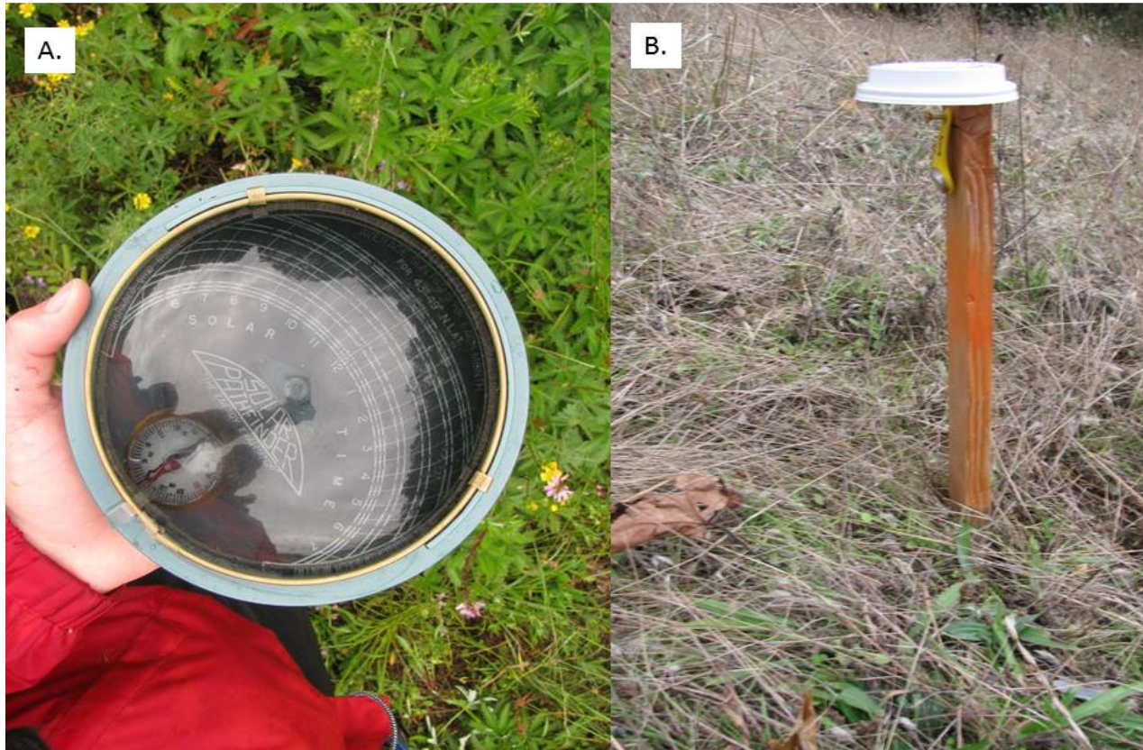
FIGURE 3. A. USING THE SOLAR PATHFINDER TO COLLECT DATA ON LIGHT AVAILABILITY. B. HYGROCHRON IBUTTONS COLLECT DATA ON TEMPERATURE AND RELATIVE HUMIDITY IN EACH PLOT EVERY 30 MINUTES.
