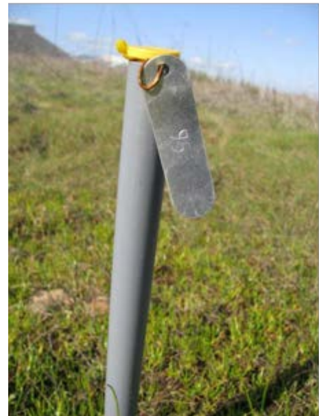
Figure 2. Example of a gray conduit post with aluminum tag used to mark 1 m 2 plot corners.
