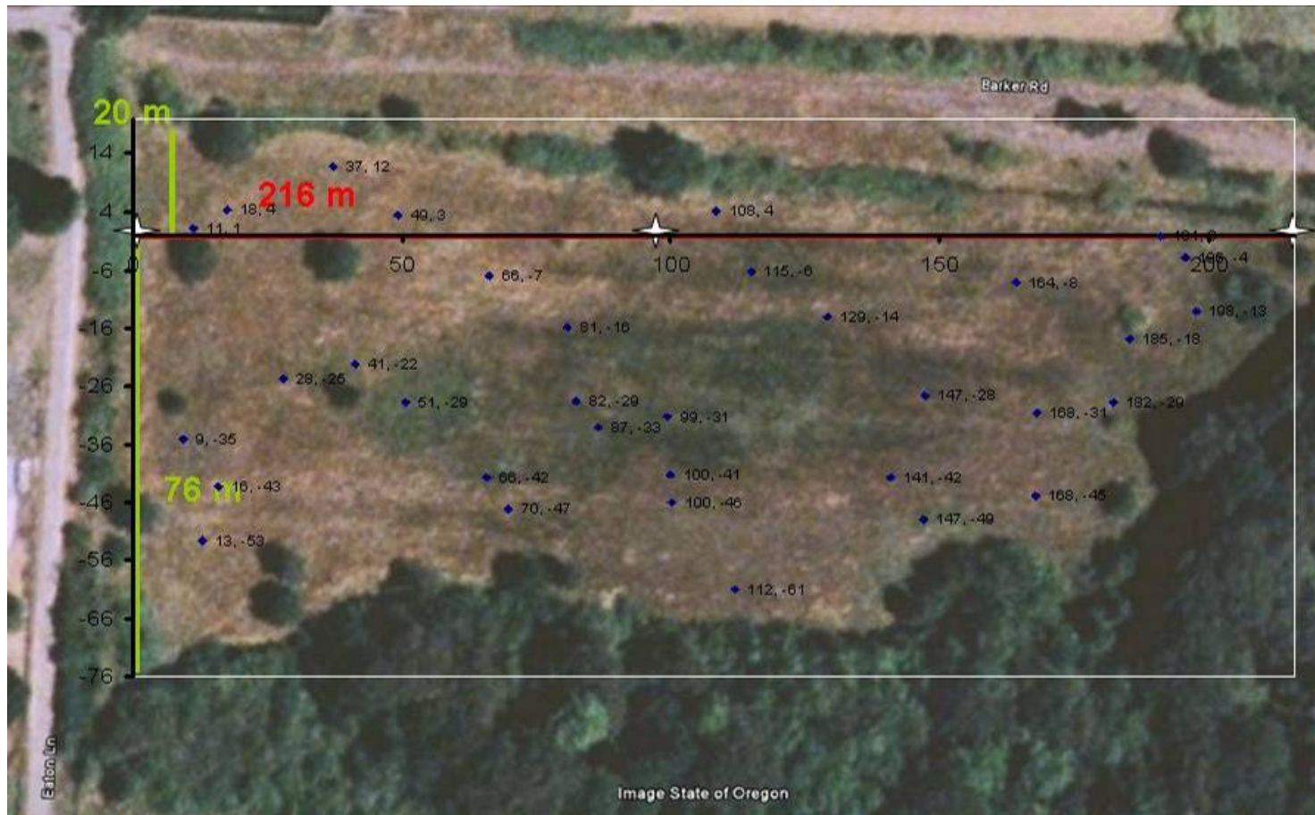
Figure 19. North Eaton upland prairie restoration site at Fern Ridge Lake. An x and y-axis were superimposed on the meadow in order to randomly select locations for sampling plots. T-posts were placed at 0, 100, and 200m on an axis running east-west. The small diamonds and coordinates represent the locations of each randomly placed sampling plot.
