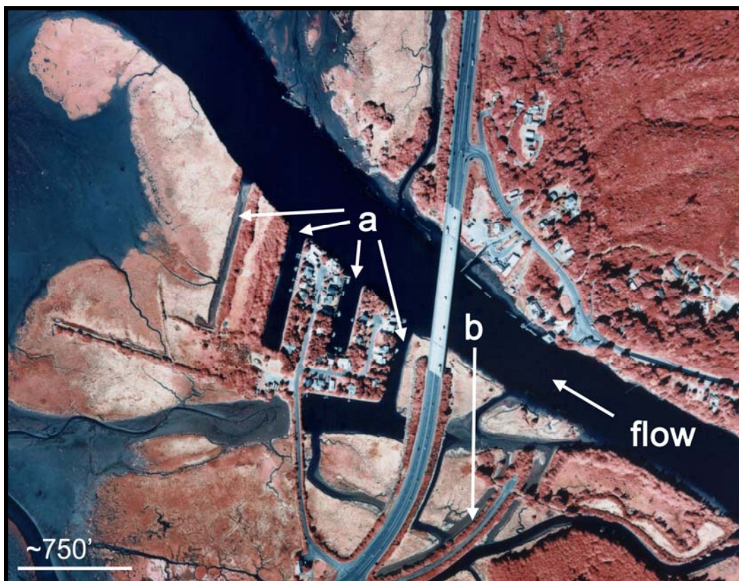
Labeled features: a = excavated boat basins with adjacent filled areas (residential development); b = spur road (old Highway 101) acting as channel armor on distributary tidal channel.
