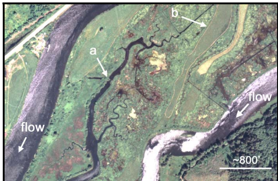
Labeled features: a = earthen dam in major tidal channel, with recent breach in center of dam; b = fence line around elongated pasture area (higher ground).
