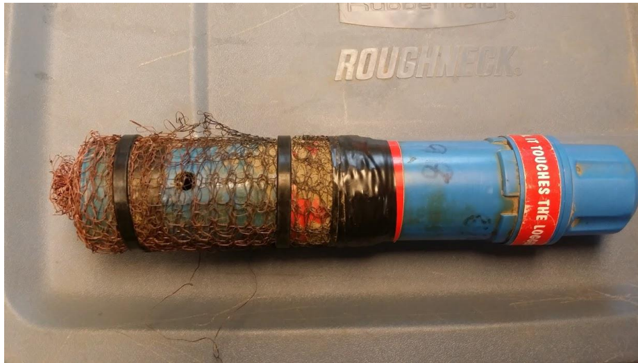
Figure 47. Odyssey salinity/temperature datalogger wrapped in copper mesh to prevent fouling.
