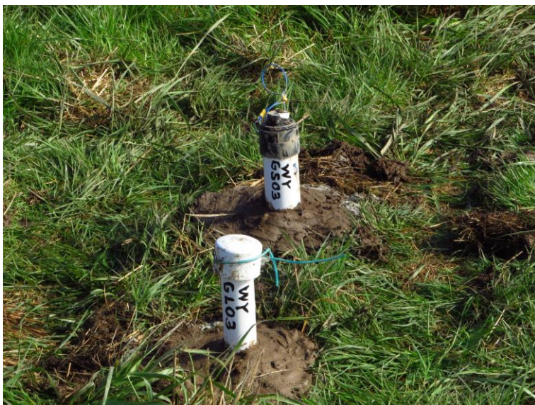
Figure 35. Closeup view of groundwater level and groundwater salinity logger installations at wetland monitoring station WY3, Wallooskee site.
