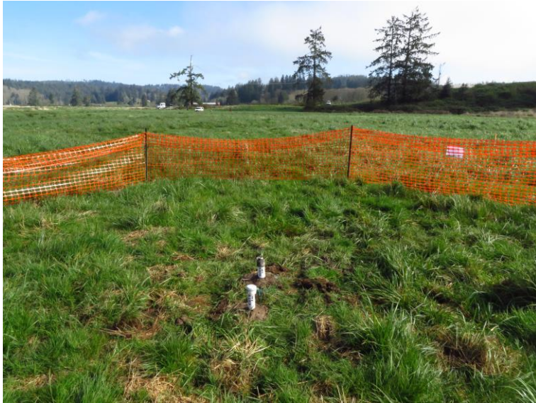
Figure 34. Groundwater level and groundwater salinity wells inside protective construction fencing at the Wallooskee site, wetland monitoring station WY3, spring 2015.
