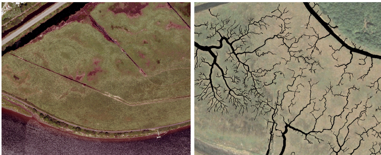
Figure 13. Channel network density comparison for an unrestored, diked former tidal wetland and a least-disturbed tidal wetland. Left: simplified channel (ditch) network in a 30.35 ha section of Waite Ranch in the Siuslaw River estuary, Oregon. Channel density is 7.95 km/km 2 ; channel length is 1.61 km. Right: dense, dendritic channel network in a 30.35 ha section of least-disturbed high tidal marsh (Millport Slough, Siletz Bay NWR; black lines show a complete field survey of channels (So et al. 2009), most of which are not visible in aerial photos. Channel density is 59.65 km/km 2 ; channel length is about 17.71 km. Figure from Brophy and Lemmer (2013).
