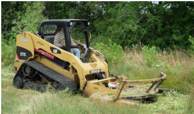
Figure 12. Mowing with skid steers is often used in prairie-savanna habitats in the fall to control woody shrub species (e.g., hawthorn or blackberry) in tight spaces or between trees in oak savanna habitats.
