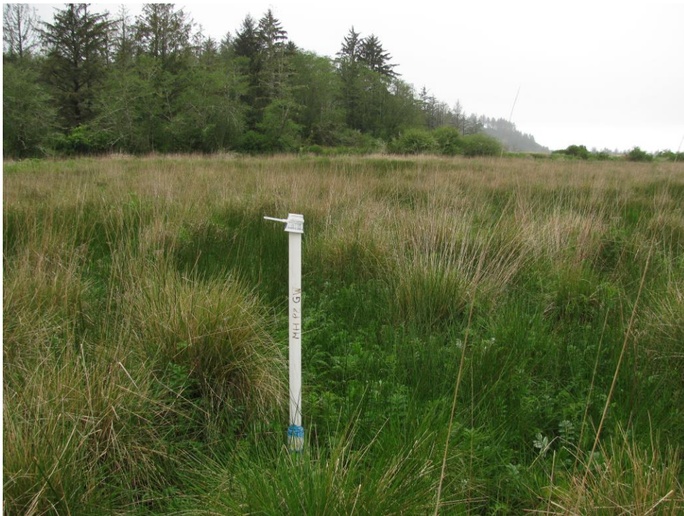
Photo 22. Groundwater well (shallow observation well) with tall riser to exclude surface tidal flows, Millport Slough Plot 2, 5/6/2009.
