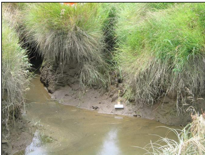
Figure 7. Water temperature reference logger located near the bottom of a tidal channel.
