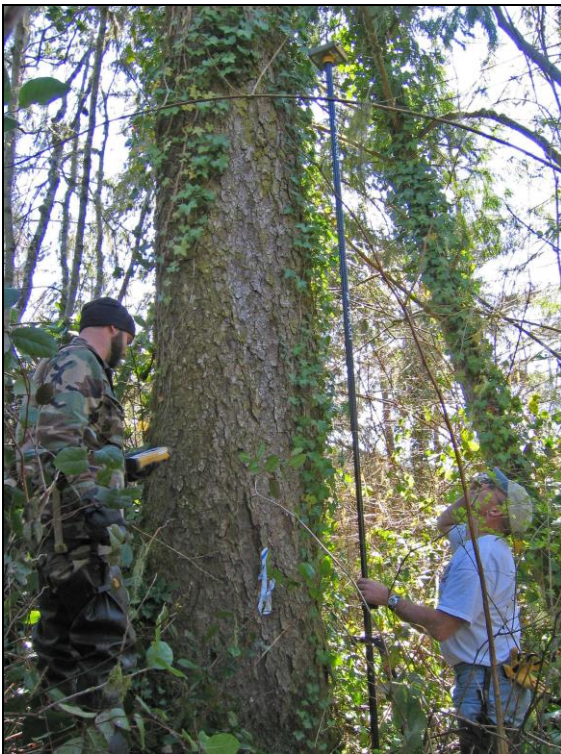
Photo 16. Doug Adams (L) and Kevin Jordan (R) of the National Geodetic Survey measuring elevations with RTK-GPS at Blind Slough Plot 1, 4/1/2008
