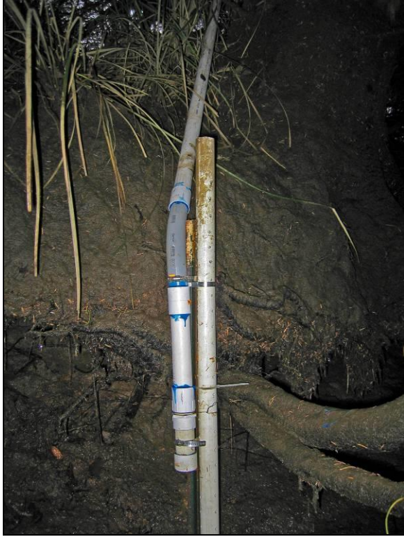
Figure 9. Side-by-side installations of a water level logger (in white PVC pipe “stilling well” at left), and vertical post deployment of several iButton temperature loggers (in vertical perforated PVC pipe at right). Deployment is located in a deep tidal channel in a forested tidal wetland in Oregon.
