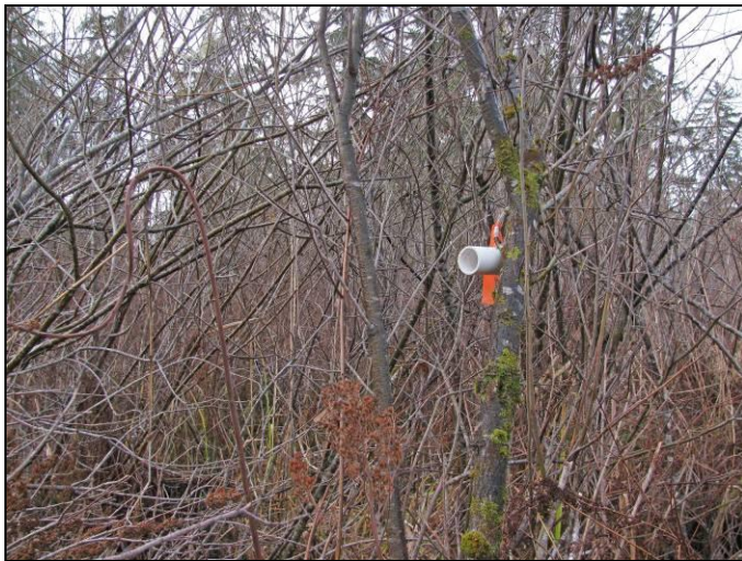
Figure 6. Air temperature reference logger wired to a shrub well above tide level, in an Oregon scrub-shrub tidal wetland.
