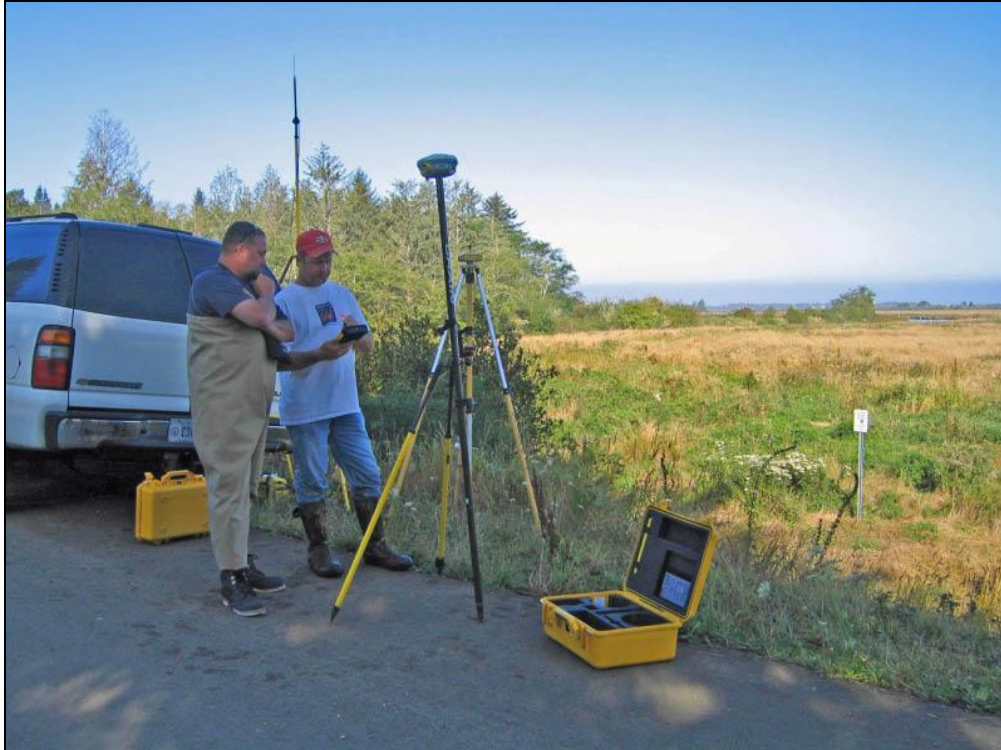
Photo 13. Steve Breidenbach and Justin Dahlberg of the National Geodetic Survey setting up RTK-GPS equipment at Millport Slough, 8/23/2007
