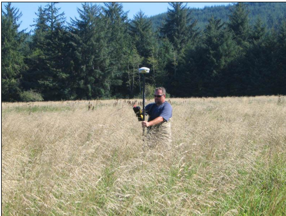
Photo 14. Justin Dahlberg of the National Geodetic Survey measuring marsh plain elevations with RTK-GPS equipment, Millport Slough, 8/23/2007
