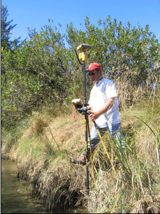
Photo 15. Steve Breidenbach of the National Geodetic Survey recording elevation of the Millport Slough HOBOT logger with RTK-GPS, Millport Slough, 8/23/2007
