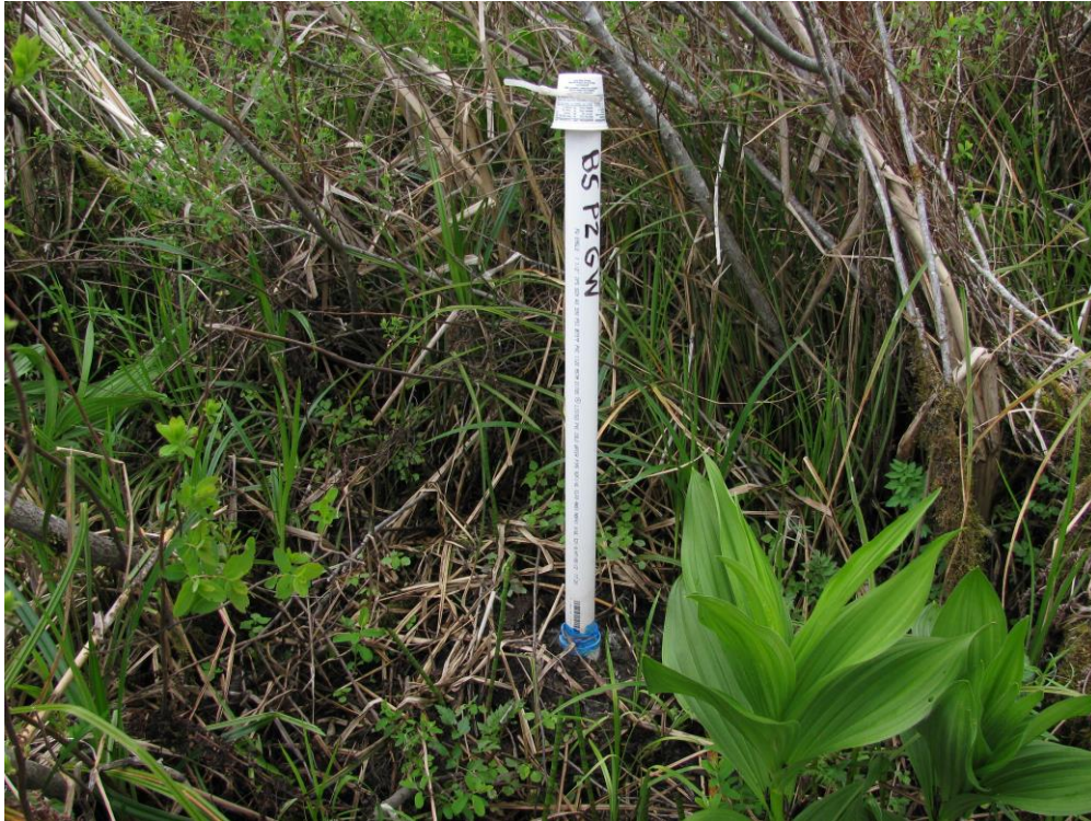
Photo 21. Groundwater well (shallow observation well) with tall riser to exclude surface tidal flows, Blind Slough Plot 2, 5/5/2009.
