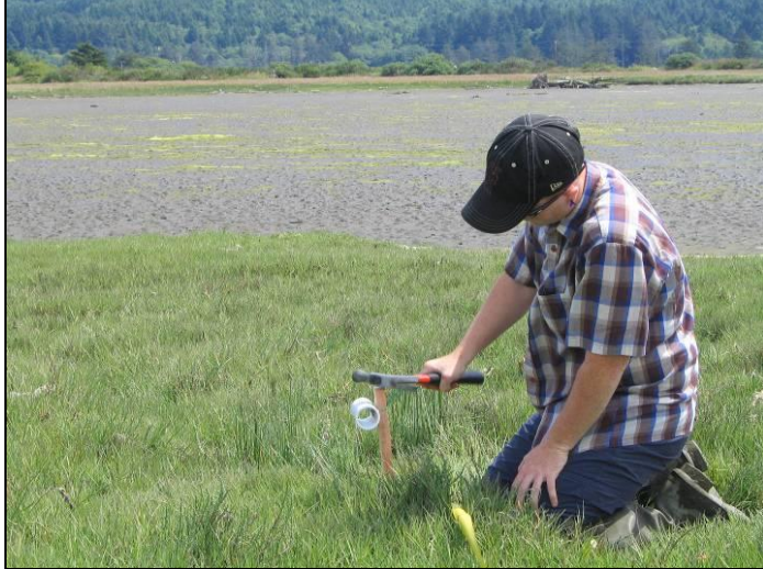
Figure 4. Deploying a surface logger inside a protective PVC sleeve. PVC sleeve and temperature logger are wired to a stake which is pounded into the marsh surface. After installation, the PVC sleeve is resting directly on the surface.
