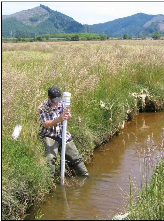
Figure 5. Deploying a vertical post arrangement in a tidal channel. The white PVC pipe contains a wooden dowel with temperature loggers attached. The pipe is wired to a metal post, which is pounded into the channel substrate.
